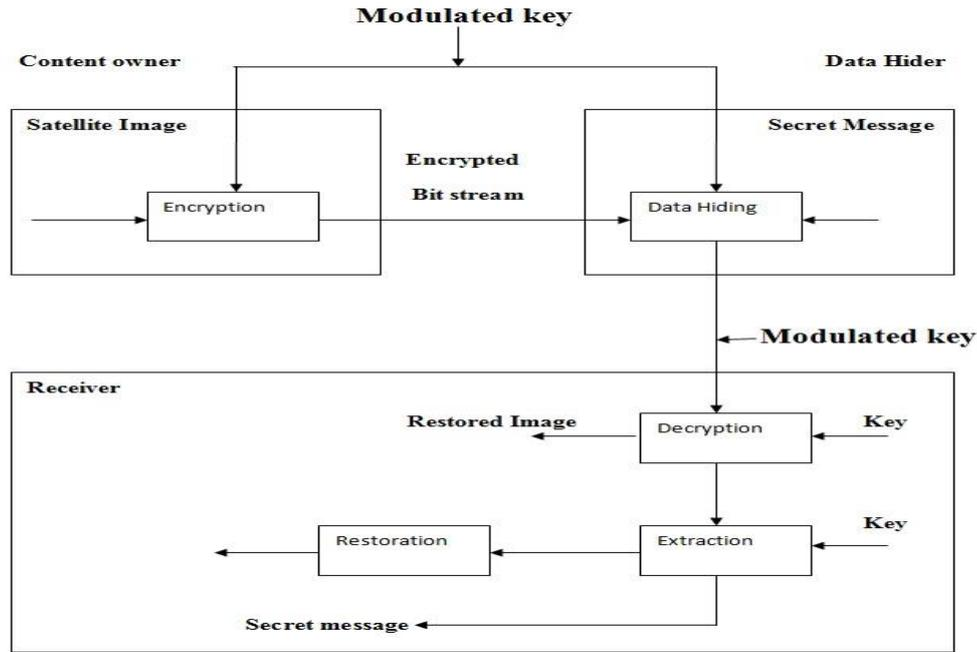
Fig. 3.1 Proposed system Architecture
